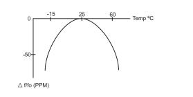
To calculate the frequency stability the parabolic curvature constant (K) is needed. For calculating the stability at  $45^{\circ}$ C?
