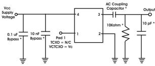
\* Required components to insure proper operation.
